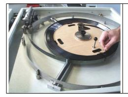
Spin rule back until it is loose in the cassette. Open one of the safety lids and tighten the rest of the rule with cable ties to the center disc.
